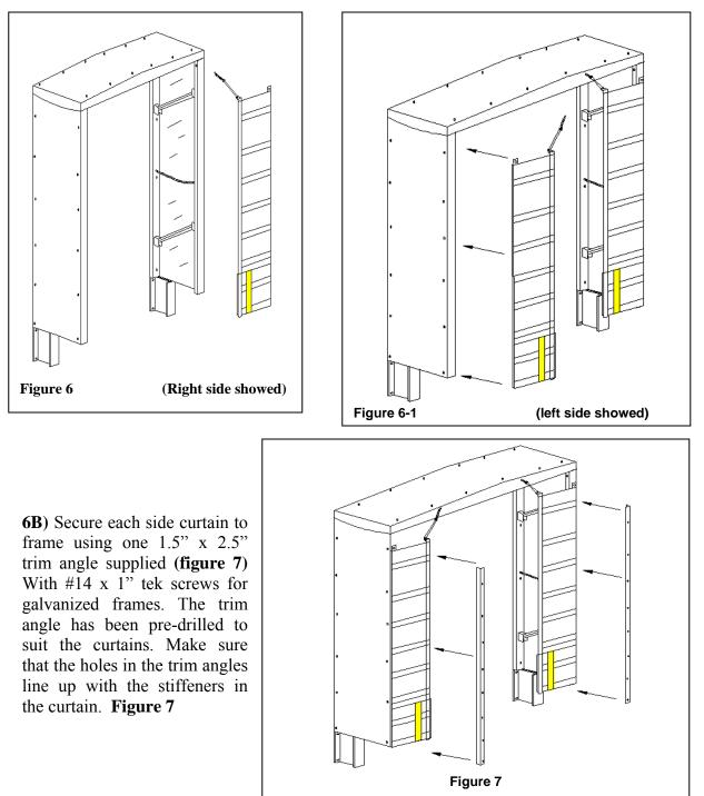
**Important Note:** You MUST ensure that the fasteners penetrate the stiffeners. It is necessary to pre-drill the stiffeners to prevent them from splitting. Also the trim angle must be attached under the perimeter cover. Figure 7-A
