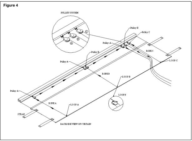
**Note:** Pulleys and loops are pre-sewn to the backside of head curtain. Lay the head curtain **FACE DOWN** on a clean surface before proceeding.
